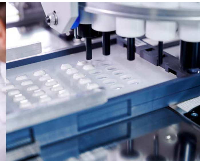
The D 3 system deblisters tablets fully automatically, safely and individually – one tablet at a time.
