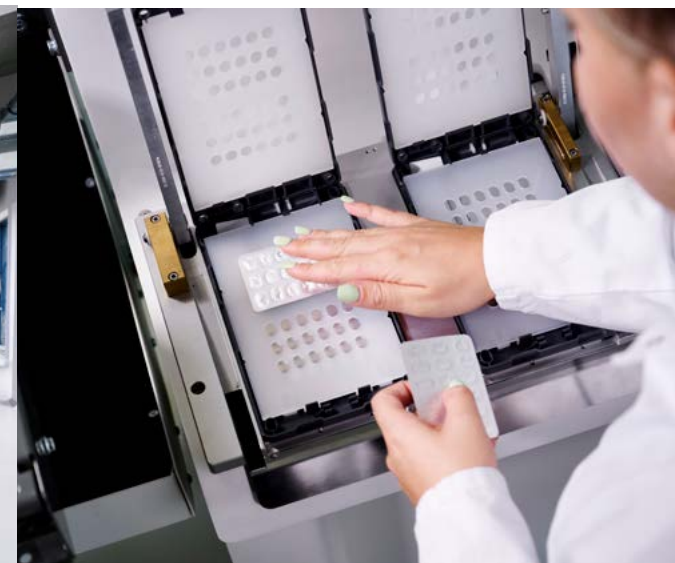
Original blister packs are being loaded into the blister carrier.
